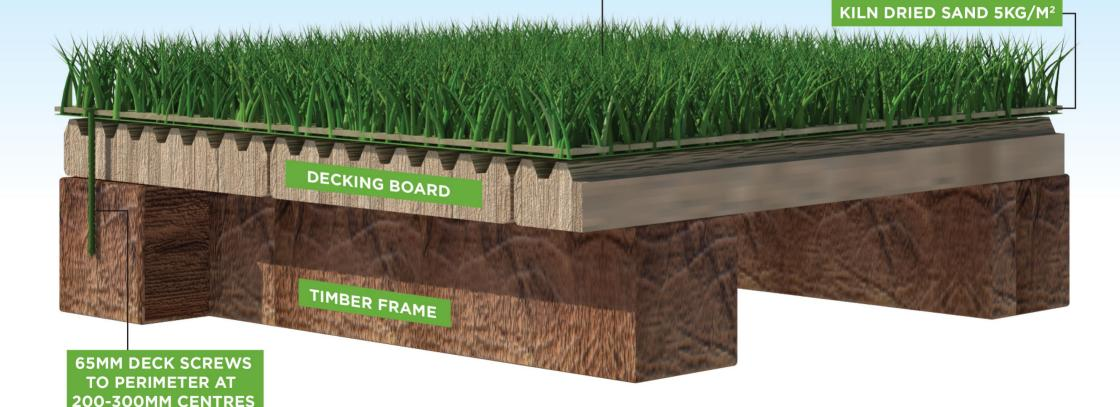
FITTED OVER EXISTING PAVING.
