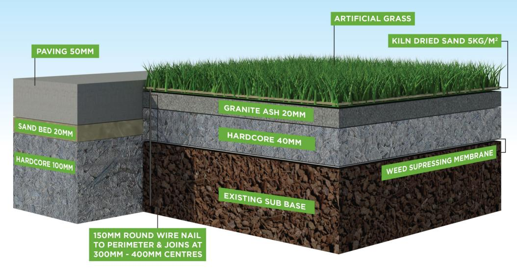
ADJACENT TO TIMBER BATON **ARTIFICIAL GRASS 65MM DECK SCREWS** KILN DRIED SAND 5KG/M<sup>2</sup> SOIL / BORDER **GRANITE ASH 20MM HARDCORE 40MM 75MM X 50MM** WEED SUPRESSING MEMBRANE **TIMBER BATON** EXISTING SUB BASE **50MM<sup>2</sup> STAKE SECURED** TO TIMBER BATON **AT 1.2M CENTRES** 150MM ROUND WIRE NAIL **TO PERIMETER & JOINS AT 300MM - 400MM CENTRES**
